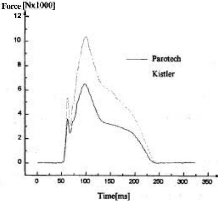
Figure 2 A comparison of force curves produced during a drop jump similar exercise. The curves were measured using a Kistler system (dotted line) and Parotech force sensors (solid line).
