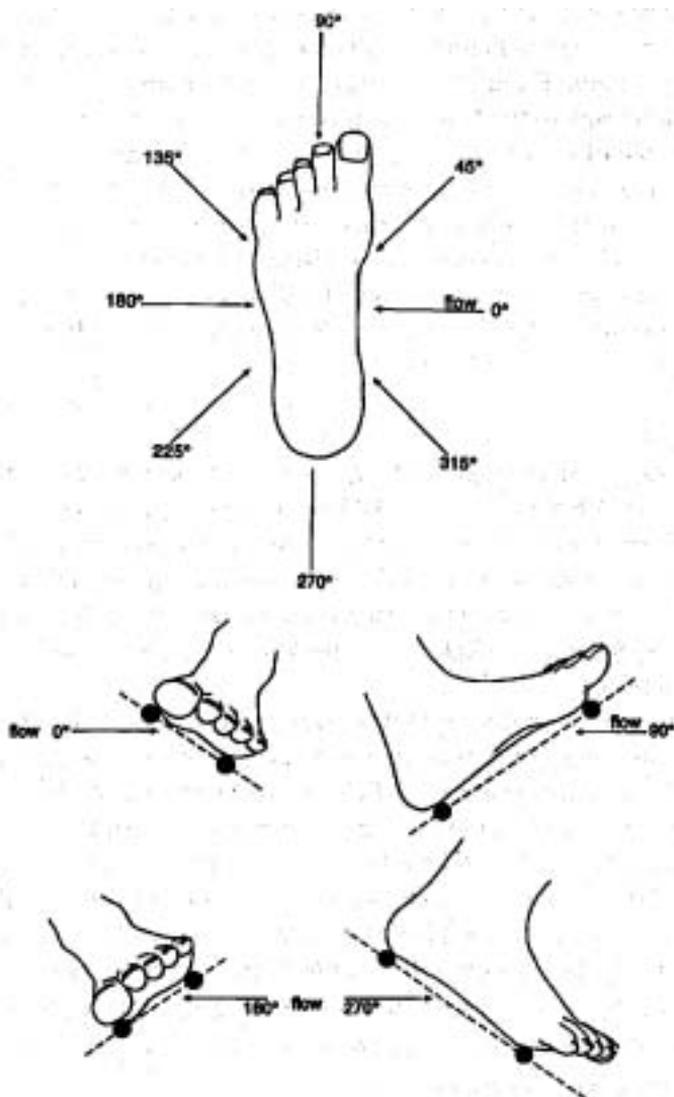
**Figure 1.** Sweepback angles (top) and the orientation of the foot with a pitch of 35 degrees for sweepback angles of 0/360, 90, 180, 270 degrees (bottom).
