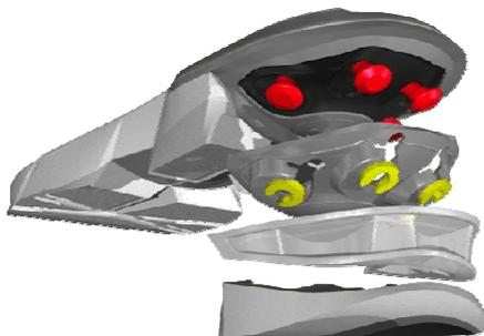
Fig. 4 Illustration of the "Ground Control System". The illustration shows from top to bottom (a) the top plate, (b) 4 springs, (c) a bottom plate, (d) spacers and (e) clear rubber sealing. With permission of adidas
