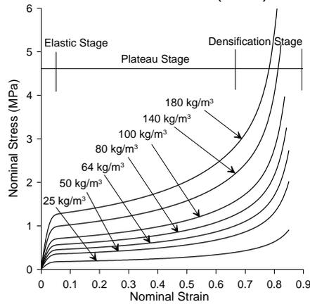
**Figure 1: Stress-strain curves for representative densities of EPS foam**
