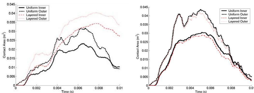
**Figure 3: Evolution of contact areas at the inner and outer surfaces of helmet liner using either a uniform liner or a layered liner: (a) Low energy impact; (b) High energy impact**
