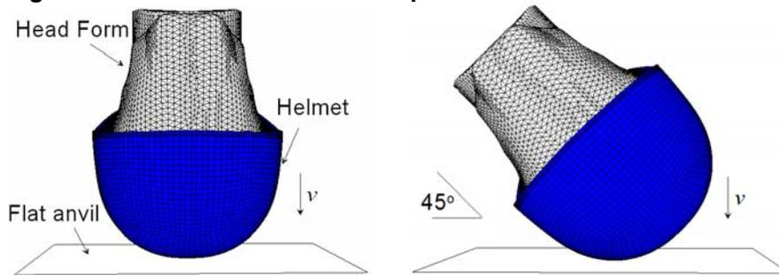
**Figure 2: Representative impact configurations (a) 45° side impact; (b) normal crown impact**
