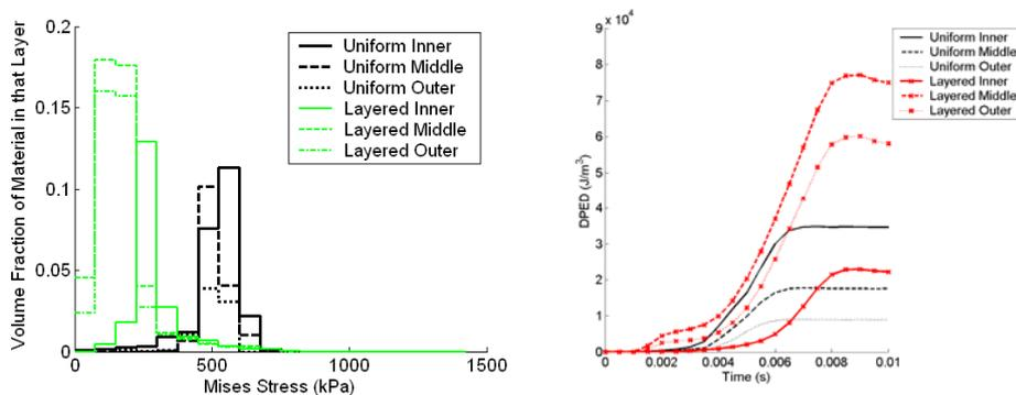
**Figure 4: (a) Distributions of von Mises stress at peak acceleration in three layers for helmet liner of uniform density and of layered density at low energy impact; (b) Evolution of average DPED in three layers for helmets of uniform density foam and of layered density foam at low energy impact**
