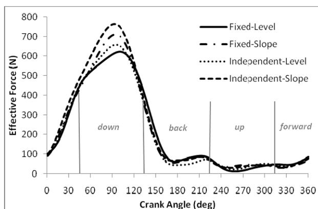
**Figure 1. Effective forces for one crank cycle of a single subject during maximal effort for 4 cycling conditions**
