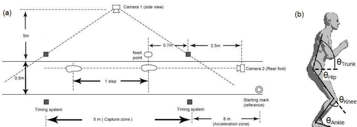
**Figure 1: (a) Experimental set up on field, drawing not to scale
