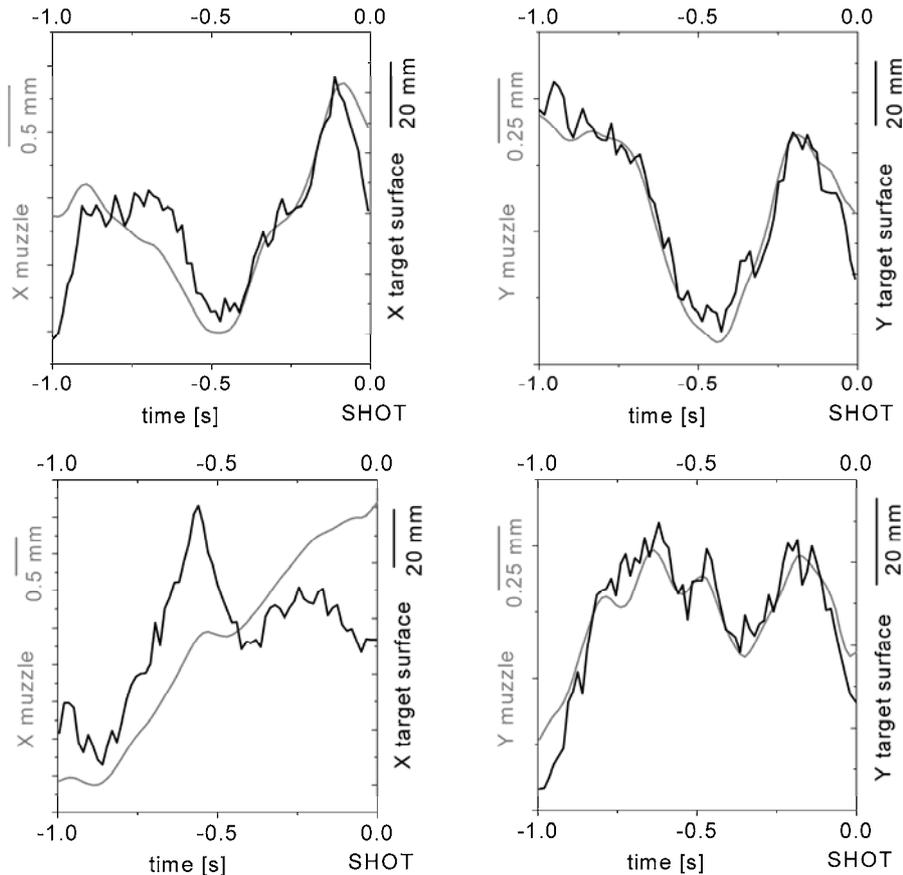
Figure 4: Sample trajectories of two shots as a function of time. Top: example shot for a high similarity in both X- and Y-direction. Bottom: example shot for a poor similarity in X-direction.
