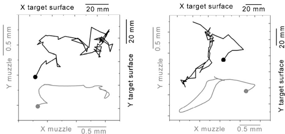
Figure 3: Sample 2D-trajectories and hits of two different shots. The muzzle trajectory in X-direction is shown mirror-inverted. Note that relative trajectories are obtained only.
