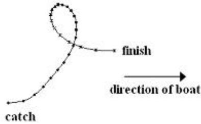
**Figure 1: Path of oar blade during the drive phase of a stroke.**
