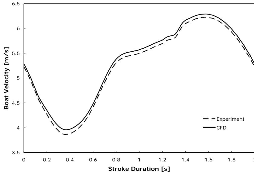
**Figure 3: Variation in boat velocity during a rowing stroke. Output when experimental values and CFD predicted values of force coefficient are used.**
