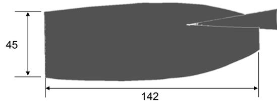
**Figure 2: Geometry of Macon blade (dimensions defined in mm).**
