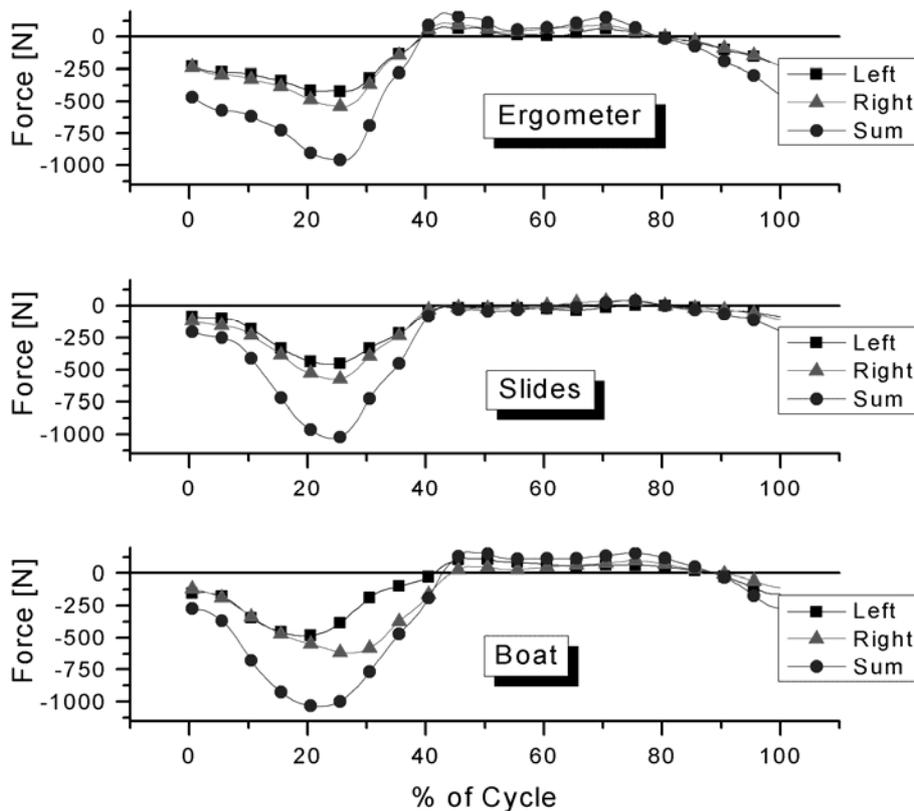
Figure 2: Horizontal reaction forces at the foot stretcher. Upper chart: static ergometer, middle: ergometer on slides, lower chart: boat. 30 strokes/min.
