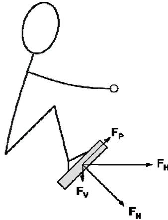
Figure 1: Reaction force components normal and parallel to foot stretcher and corresponding horizontal and vertical forces.
