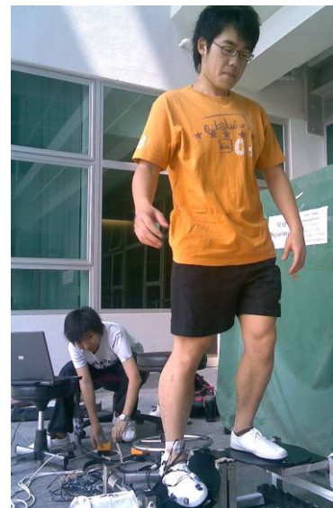
Fig 1: A subject performing simulated sprain motion on a mechanical ankle sprain simulator
