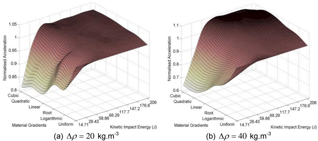
**Figure 2. Surface plots of normalised (against uniform foams) peak accelerations of five material gradients across a range of striker impact energies. Significant reduction of peak acceleration is seen in the low energy regions of the plot.**
