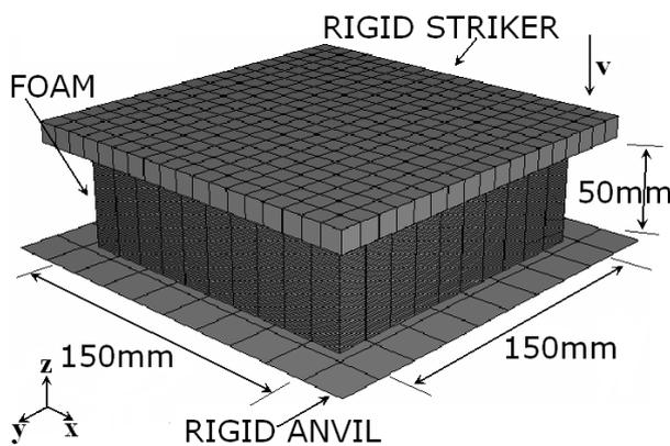
**Figure 1. Modelling of the FGM is achieved by approximating a specimen with a continuous variation in material properties as fifty discrete, finely meshed element layers through the thickness, with a unique  $\sigma - \varepsilon$  curve associated with each layer along the z-direction.**
