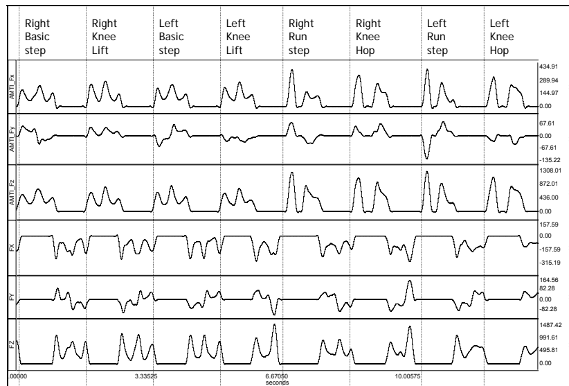
Figure 1: Identification of a sequence of Step movements in the horizontal and vertical components of the GRF, during the ascending (AMTI Fx, Fy & Fz) and descending (Fx, Fy & Fz) phases of the movements performed at 140 bpm (one representative subject).
