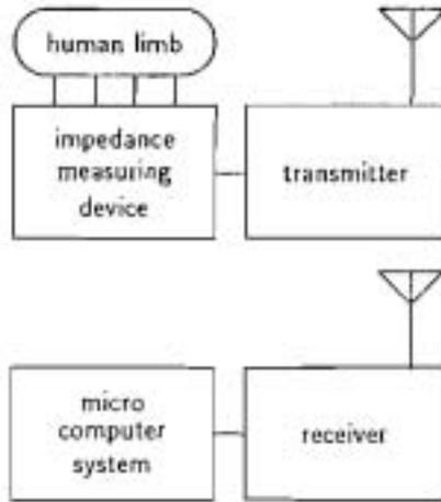
Fig.1 Impedance measuring system.
