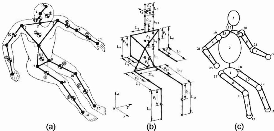
Figure 1 - Three-dimensional biomechanical model: (a) Human body; (b) Local coordinate frames; (c) Contact surfaces.
