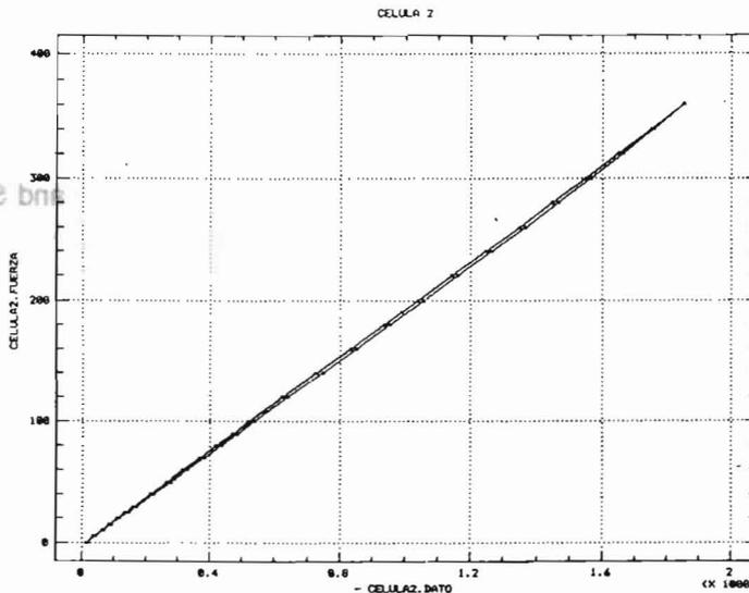
Figure 1. Detailed representation of the components of the uniaxial load cell system with its calibration curve.
