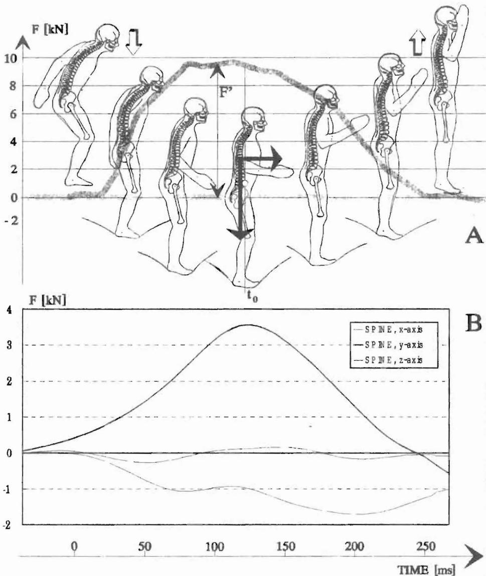
**Fig. 7** Representation of forces exerted in the landing phase in trampolining gymnastics
