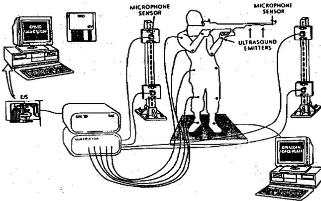
Fig. 1. The measurement chain set up.
