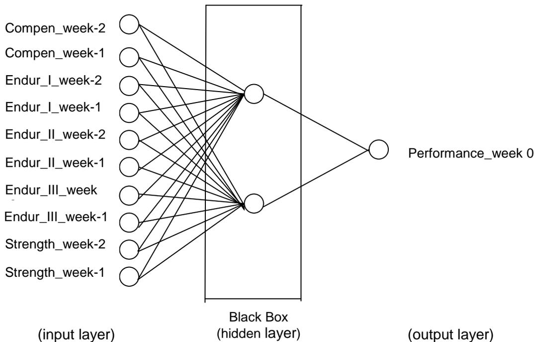
**Figure 2 - The structure of the multilayer backpropagation net ('multilayer perceptron', DataEngine Inc., Aachen, Germany) used to model the interrelation between the training input data and the performance output data.**
