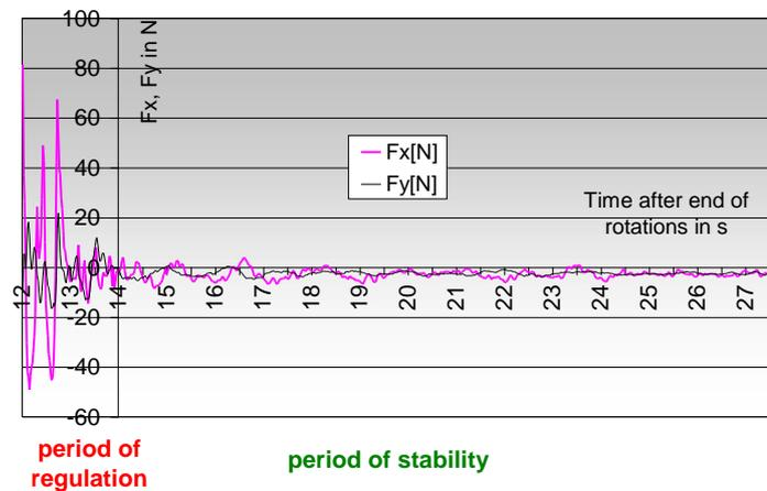
**Figure 3 - Example of a force-time curve ( $F_x$ ,  $F_y$ ) after 10 rotations in the simulator.**
