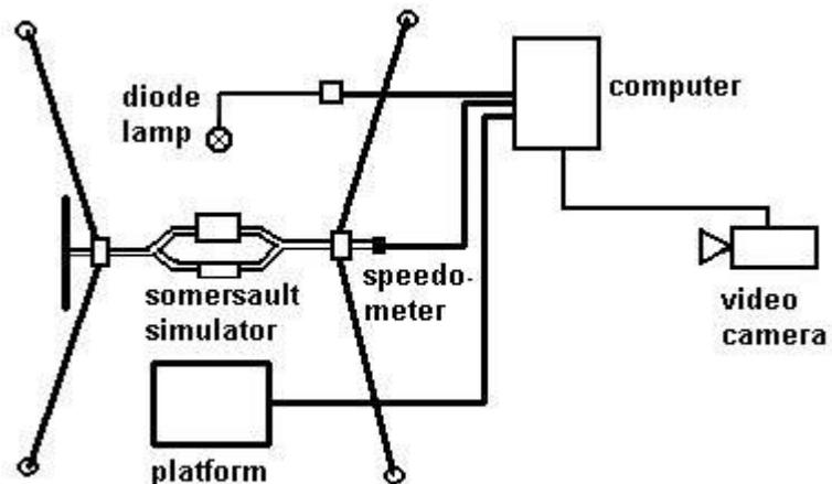
**Figure 2 - Schematic of the somersault simulator.**
