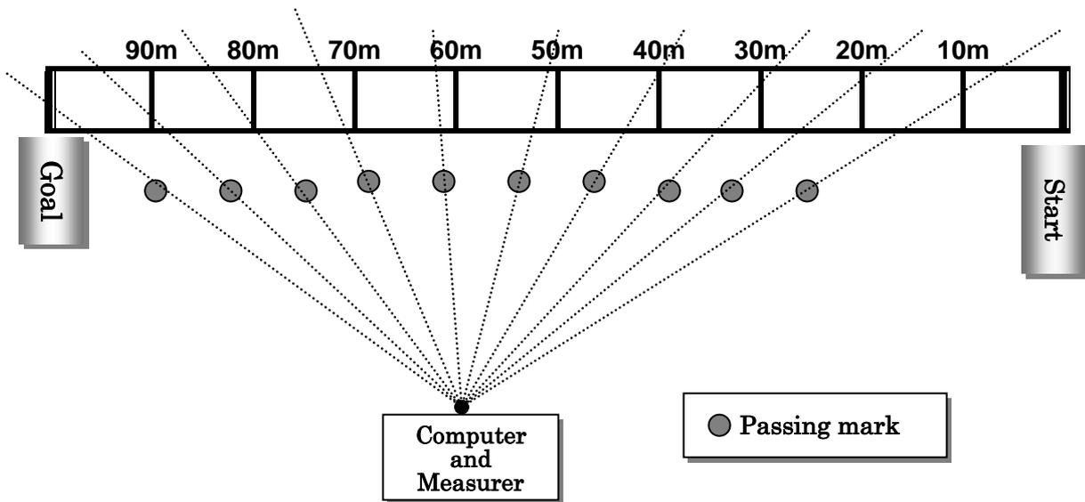
Figure 1 - The experimental straight lane for the measurement of the 100m dash is shown. The lane was divided equally into 10 sections. Each passing mark was placed on an extension line from the measurer to a passage point of each section.
