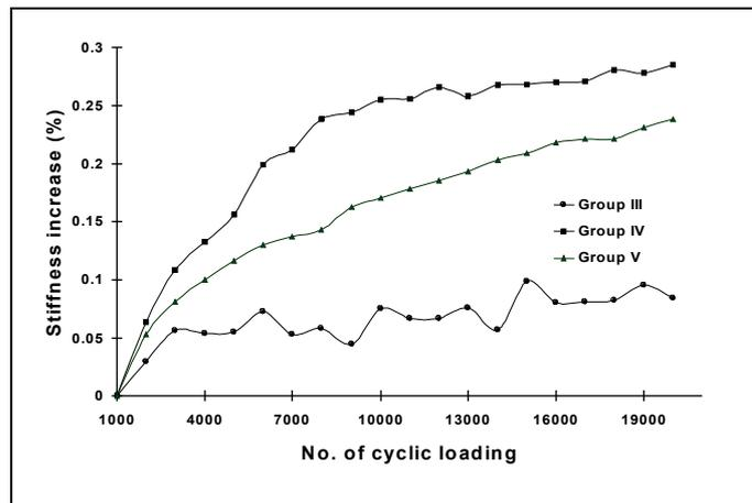
**Figure 2 - Average stiffness change of specimens during cyclic loading in groups III, IV and V. Stiffness significantly increased during initial 5000 cycles.**
