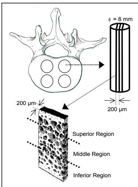
**Figure 1 - Schematic diagram of experimental design for measuring microfracture after mechanical fatigue testing.**
