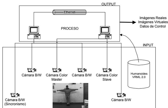
**Figure 1 – The setting of 6 configurable points of view.**
