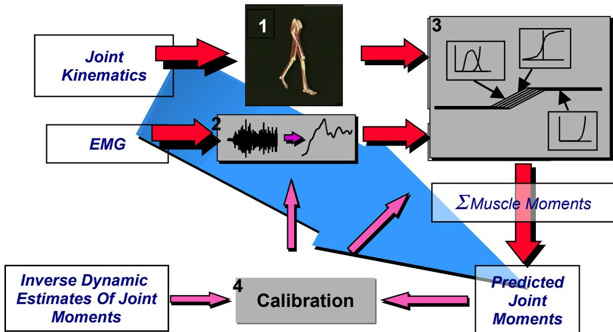
**Figure 1 - Schematic of the EMG driven knee joint model showing the sub-components; 1) anatomical model, 2) EMG-to-activation model, 3) muscle model, and 4) calibration.**
