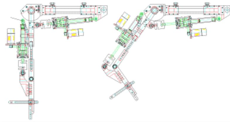
**Figure 1: The driving part of the robotic gait trainer**
