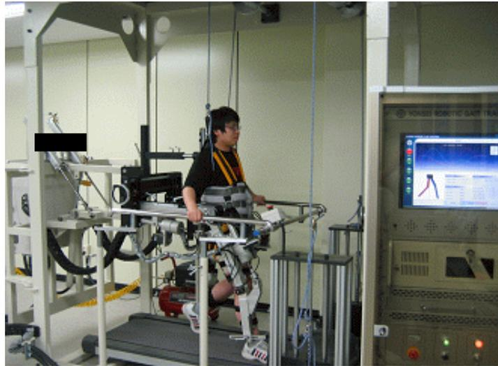
**Figure 5: Developed robotic gait trainer**
