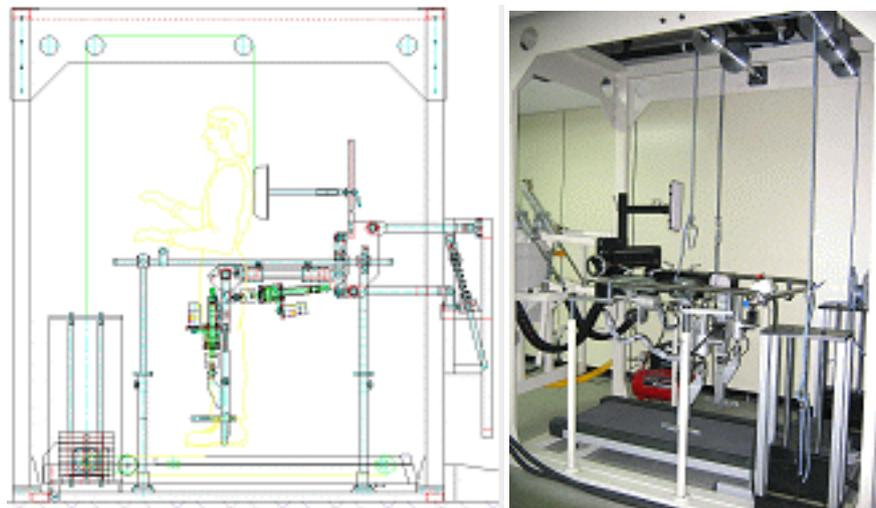
**Figure 2: The weight support system of the robotic gait trainer**
