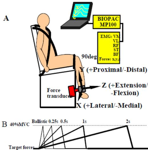
Figure 1. Schematic representation of experimental setup (A) and target force trajectories (B) in the present study
