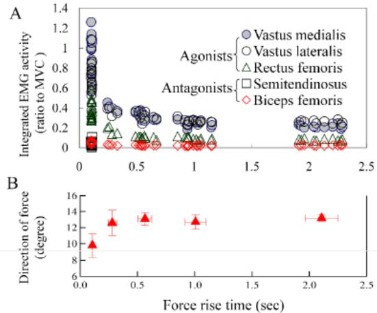
Fig. 3. Integrated EMG activity (A) and direction of resultant force on z-x plane (B) as a function of force rise time
