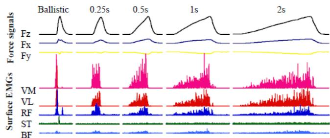
Fig. 2. Representative recordings of three components of force signals and surface EMG activities on thigh extensor and flexor muscles at five different force rise times
