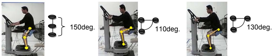
Figure 1: The angle definition of dynamic movement and static posture on vibration platform.
