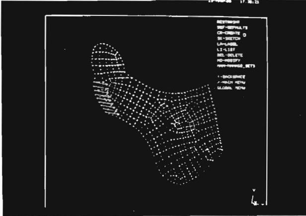
Arrows to the left represent force vectors. Arrows to the right are restraints for the x- and y-directions.
