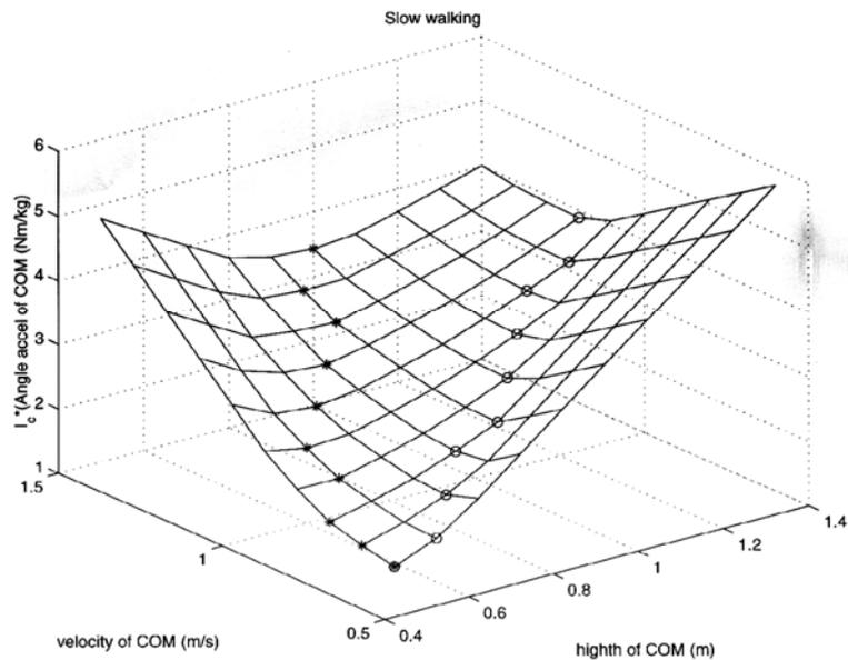
**Figure 2** Simulation of the stability of loaded walking at slow walking.
