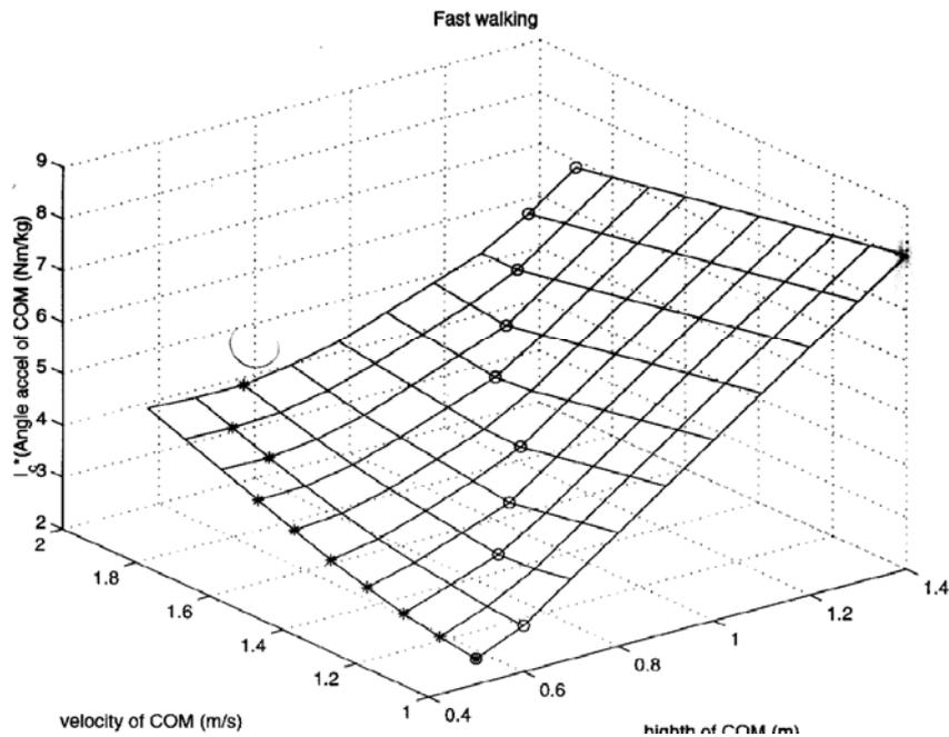
**Figure 3** Simulation of the stability of loaded walking at fast walking
