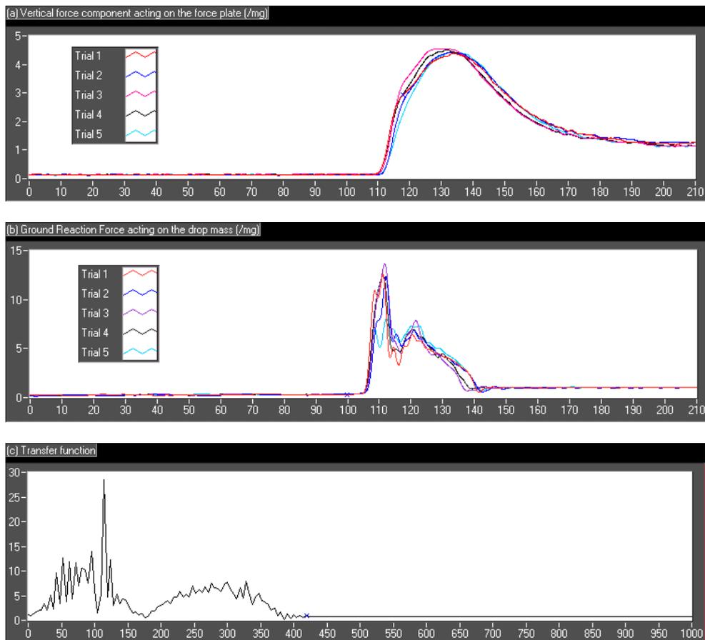
**Figure 1.** Calculating the transfer function  $P^{-1}(\omega)=Y(\omega)X^{-1}(\omega)$  for a drop mass of 3.86kg, a release height of 0.1m, and a sand depth of 0.1m. (a) The normalized vertical reaction force measured by the force plate against time (ms). (b) The
