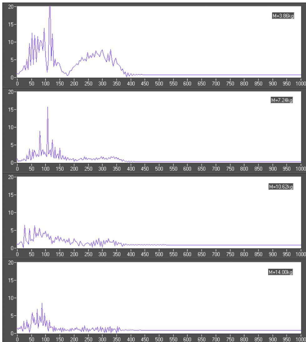
**Figure 2.** Average transfer functions against frequency (Hz), calculated for different drop masses  $M$ , which are released from a constant height of 0.1m. The sand covering the force plate is dry and uncompacted, and its depth is 0.1m in every case.
