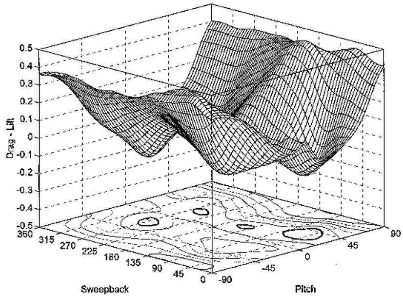
**Figure 3:** Difference in magnitudes of drag and lift coefficients obtained from a resin model of a swimmer's hand with adducted thumb
