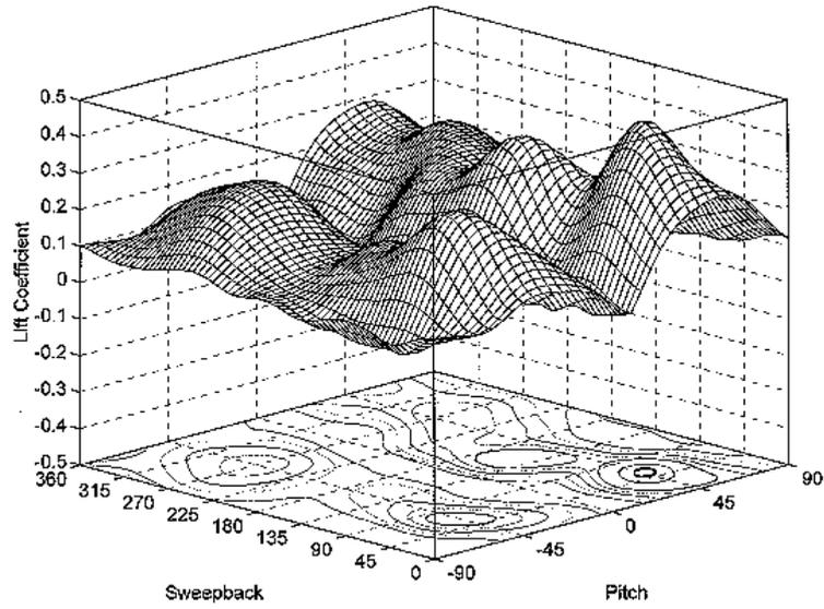
**Figure 2:** Lift coefficients obtained from a resin model of a swimmer's hand with adducted thumb
