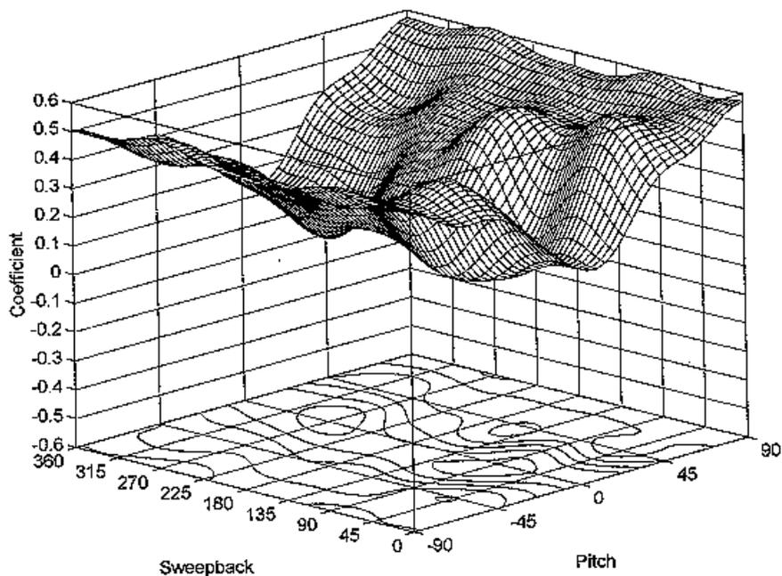
**Figure 1:** Resultant of the lift and drag coefficients obtained from a resin model of a swimmer's hand with adducted thumb.
