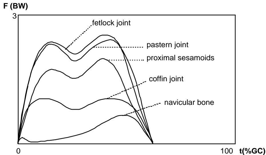
**Figure 3** — Joint forces, results of the model
