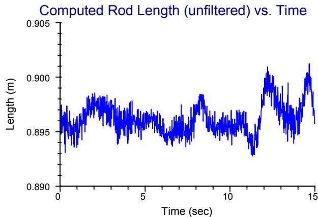
Figure 1: Computed length of a 0.9 meter rod as it moved through a 15m x 4m x 2m volume
