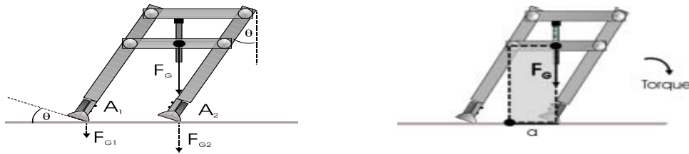
Fig. 2a: The model with defined angle of canting \theta shown on the plane Fig. 2b: Visualization of the torque
