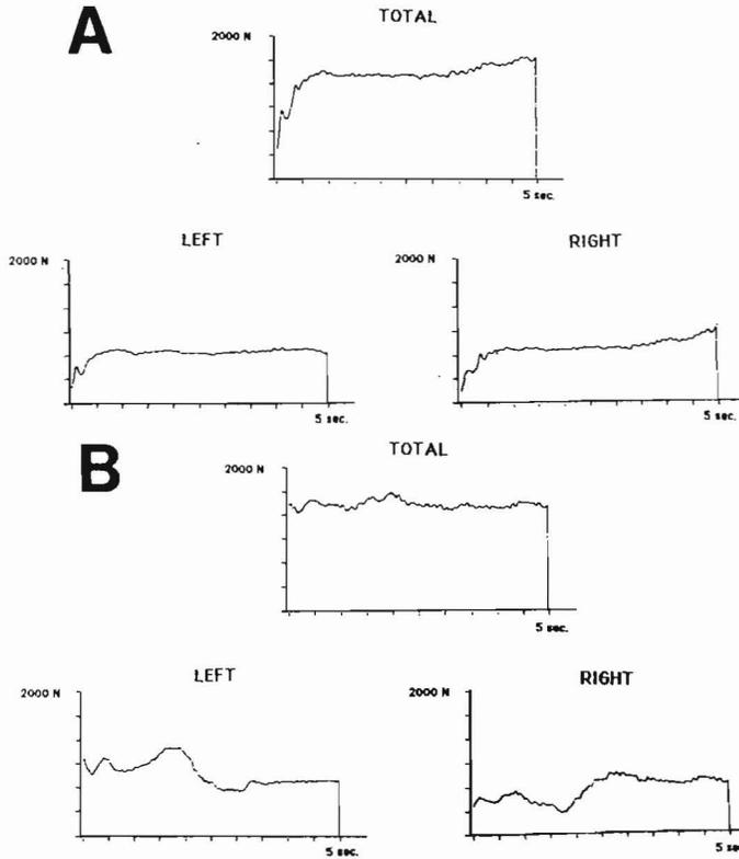
Figure 5 - Time course of the horizontal ground reaction forces exerted by the subject of fig. 3 during test A and B. For each test are shown the forces exerted by each foot and their sum.
