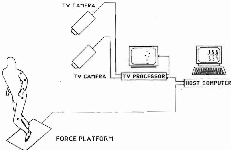
Figure 1 - ELITE system for kinematic analysis of sport performances.
