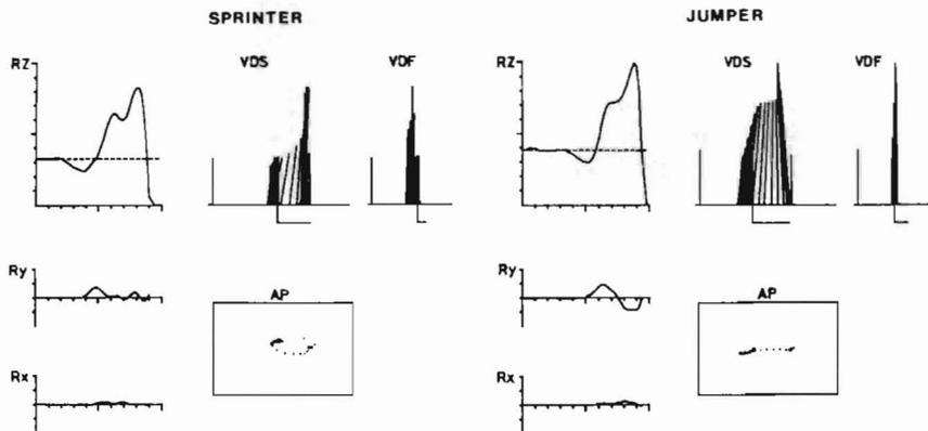
Figure 8 - Patterns of ground reaction forces measured during vertical jump of sprinter and high jumper. Rz, Ry, Rx are the time courses of the three components, VDS is the vector diagram projected on the sagittal plane (forefoot of the athlete on the left) VDF is the vector diagram projected on the frontal plane (right side of the athlete on the left), AP is the time course of application point on the force plate plane.
