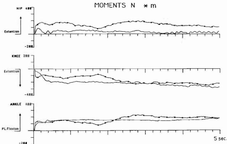
Figure 6. Hip, knee and ankle moments of the right limb measured during the push of a rugby player. Dark lines are from condition A, dark-dotted lines are Condition B.
