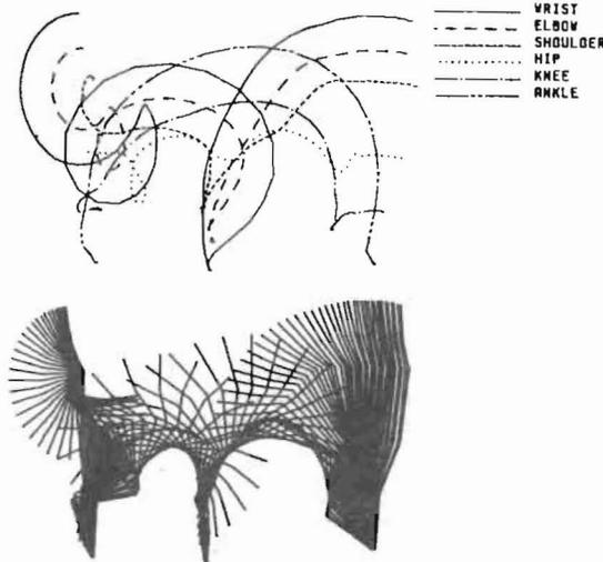
Figure 10 - Trajectories of the markers recorded during the backward somersault of a gymnast and stick representation of the body position. Start position on the left.
