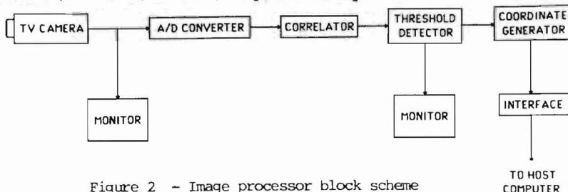
Figure 2 - Image processor block scheme
