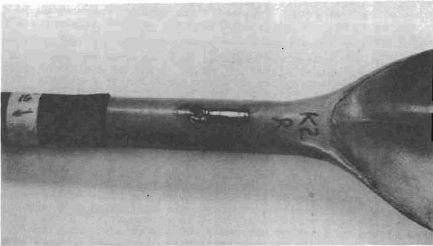
Figure 4. Strain-gauge location - kayak paddle.
