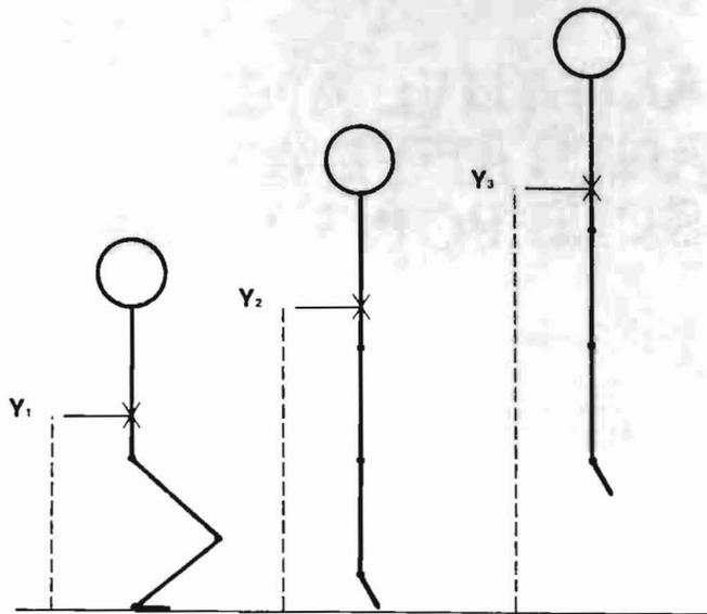
Figure 1. Three positions involved in the analysis of a vertical jump. These positions are  $Y_1$ , the lowest crouched position;  $Y_2$ , the extended position just as the body releases from the floor; and  $Y_3$ , the highest point of the jump.
