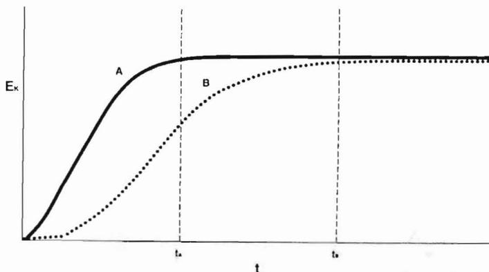
Figure 2. Two runners A and B obtain the same kinetic energy  $E_k$ , but runner A does it in the shorter time  $t_a$ , while runner B does it in longer time  $t_b$ . Runner A, therefore, is by definition the more powerful of the two.
