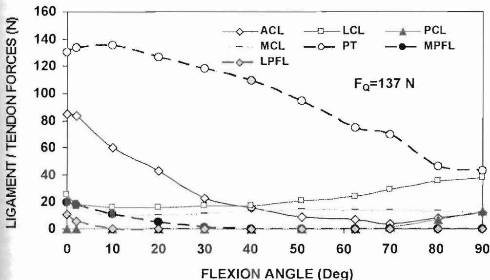
Figure 2: Computed forces in joint ligaments and patellar tendon at different flexion angles under quadriceps force of 137 N.
