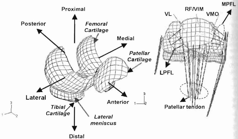
Figure 1: The knee joint finite element model showing cartilage layers, menisci, ligaments, patellar tendon and quadriceps muscles. Bony structures are not shown.
