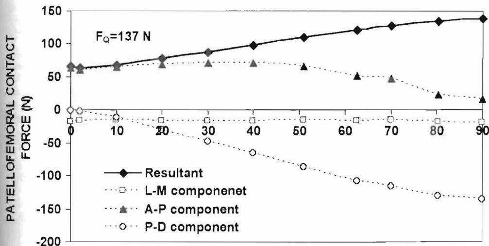
Figure 3: Resultant patellofemoral contact force and its components in different anatomical directions as a function of joint flexion under 137 N constant quadriceps muscle force.
