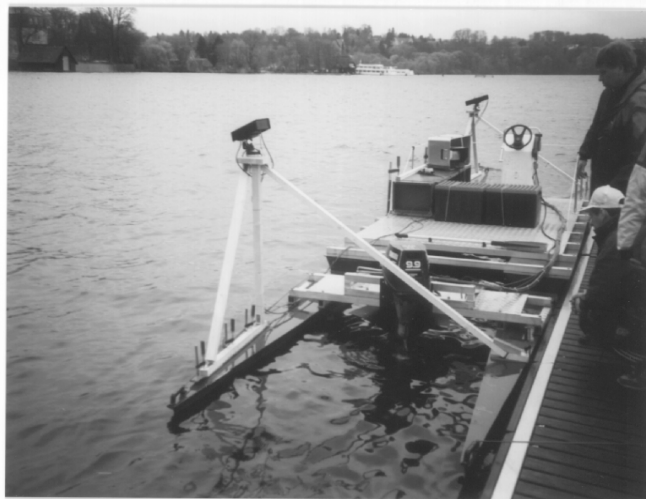
Fig. 2: Catamaran for 3D measurements
