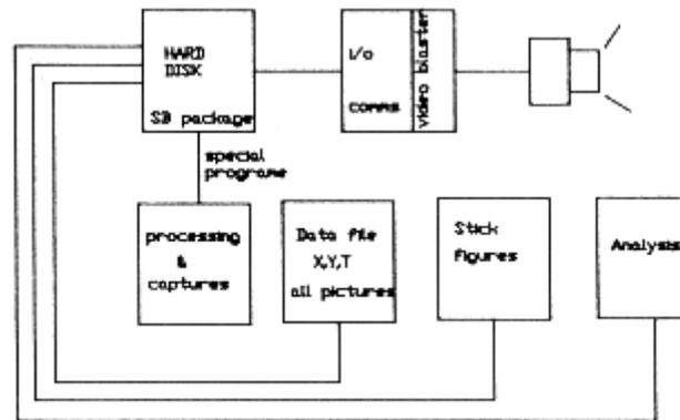
The method of analysis is similar to that used by cinematography. The actual system is composed of a video camera, a video blaster, a computer, a computer program Figure (1).
