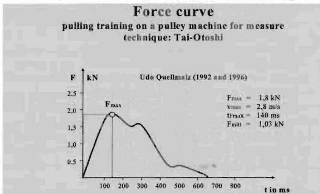
**Figure 3** Characteristic force-time curve on an arm pulley machine measurement unit for the Tai-Otoshi technique of **Udo Quellmalz** (1992 and 1996).
