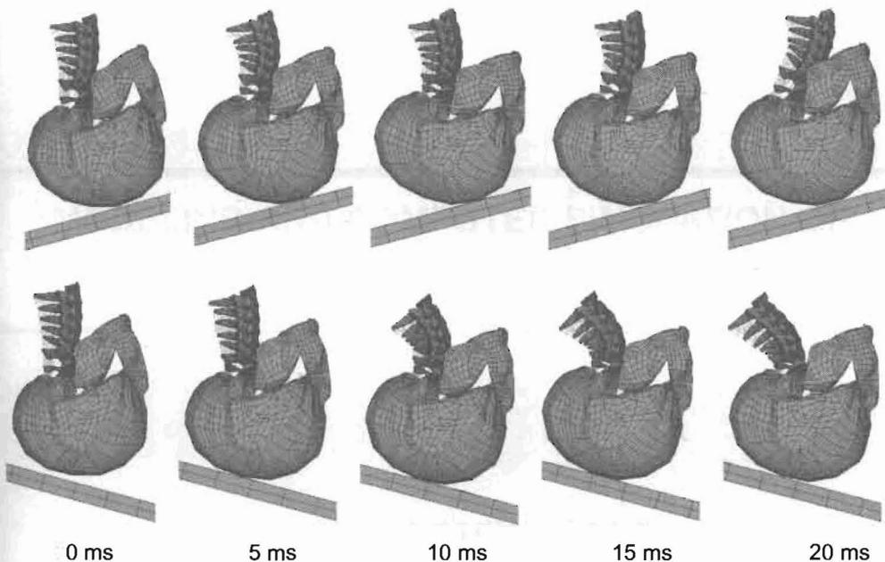
**Figure 3 Predicted response of the neck in the near-vertex impact.**
