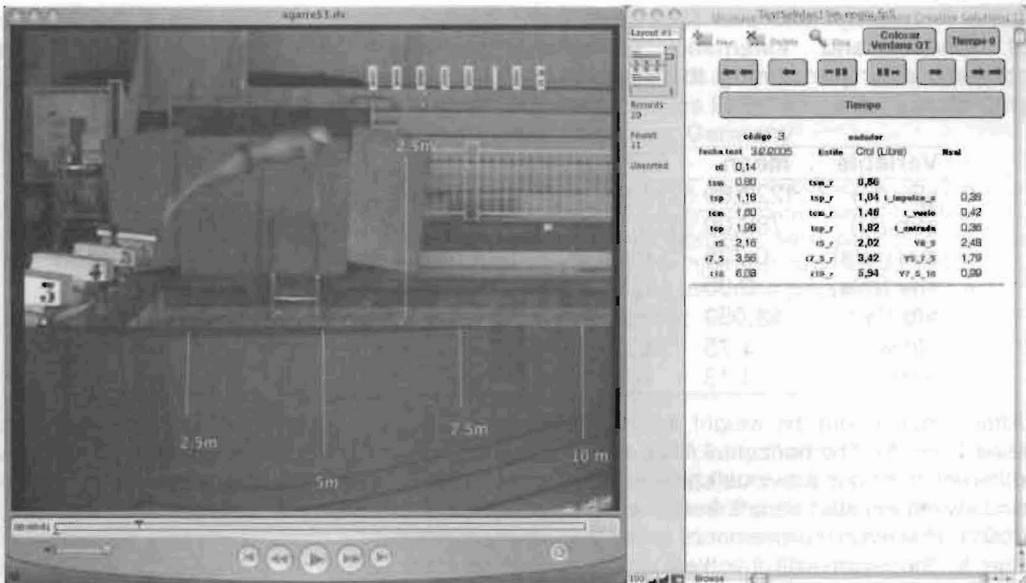
**Figure 1** A descriptive view of the digital video (Quicktime .dv format) controlled from the data-base (Filemaker 6.0) thanks to scripted buttons. The biggest button inserts the digital time code in the specific data base field. The rest of the buttons control the video advance and video window position. The distance references are included in the video window; they were drawn on the operative system (Mac OSX 10.3.8) desktop using the Ultimate Pen™ application.
