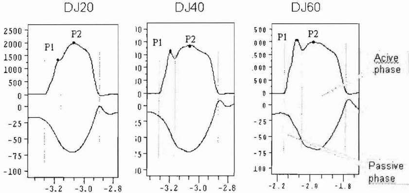
Figure 1: This is a representative figure of ground reaction force of DJ20, DJ40 and DJ60. P1 (peak force 1) is the passive force and p2 (peak force2) represents the active force. The slope between P1 and P2 is the rate of force developed between passive and active force (PARFD).
