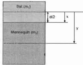
Figure 5: Schematic of the analytical model of blunt impact interaction. Variables  $x$  and  $y$  are defined as the location of the centre of mass of the bat and mannequin respectively, relative to a stationary reference frame.
