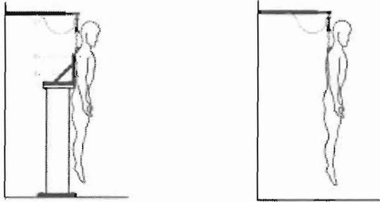
Figure 2: Restraining modes of HII: (a) Constrained: mannequin maintained suspended throughout the impact with its back blocked by a rigid column (b) unconstrained: mannequin in free fall during impact.
