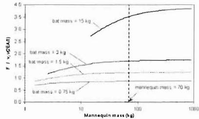
Figure 4: Peak normalized force values as a function of mannequin and bat masses.
