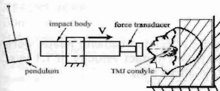
**Figure 2** Schematic diagram of the impact test of human cadaver heads. The impact forces were along the chin and vertically to the junction line of the right and left condyles.
