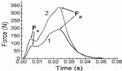
**Figure 3** The impact force-time curves upon the chins of human cadaver heads were two peaks ( $F_s$  and  $F_p$ ) profiles. Line 1 corresponds to the impact velocity of 1.1 m/s, while line 2 to 1.6 m/s. The mass of the impact body is about 6 kg.
