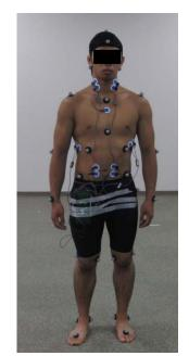
Figure 2: Placement of reflective markers and EMG electrodes.
