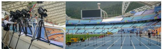
Figure 1: Camera setup on the stadium (left) and DLT calibration process of 40-70 meter capture volume (right).
